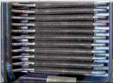
*Finned tube convection section custom engineered to improve heat transfer efficiency and allow for compact space.*
