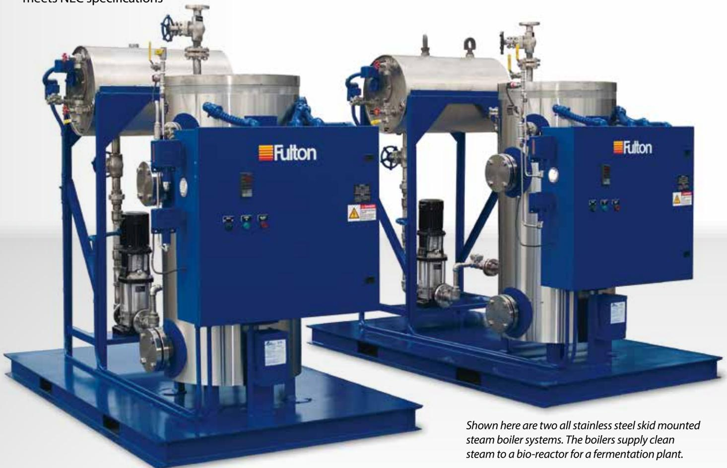
*Shown here are two all stainless steel skid mounted steam boiler systems. The boilers supply clean steam to a bio-reactor for a fermentation plant.*
